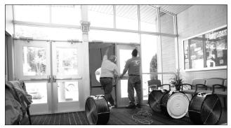
from outside the building can show patterns of air leakage. Energy saving potential is analyzed using EC 128/ALCAP software.
